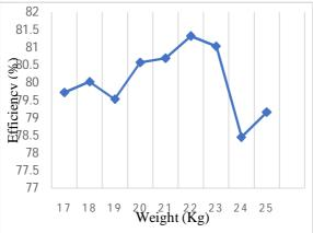
The optimal power output is obtained at a weight of 22kg which is 81.35% efficient having the power output of 0.4W for an input of 0.5W. So the mass of 22kg is selected for the system.
